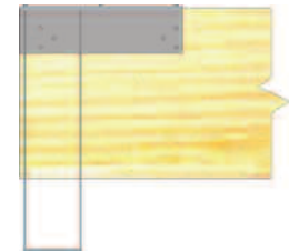
Typical LBH hanger top flange offset, right shown
